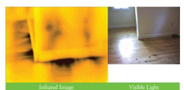
The bright yellow shows the hotter warm floor and insulation. The darker spots reveal the leaks from under the baseboard and the loss of heat through the studs.
